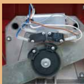
Perfect movements thank to three limit switches
